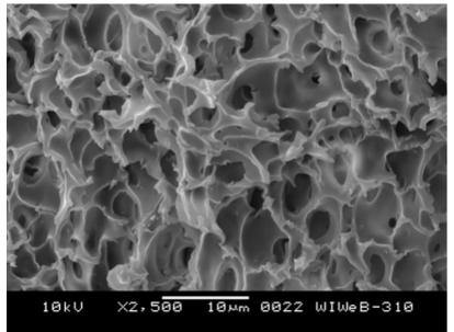
Photo enlarged 2500 times of a microporous membrane:
